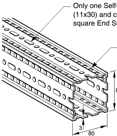
Only one Self-forming Screw FLS 80 pass-through the elongated holes (11x30) and connect into the Framo elements within the box section, e.g. square End Support to WBD F 80, octagonal End Support to STA F 80.
